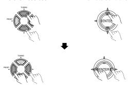
5. Use the ▲ and ▼ cursor buttons to select "Front L/R" and then use the ◄ and ▶ cursor buttons to select the front speaker setting.
